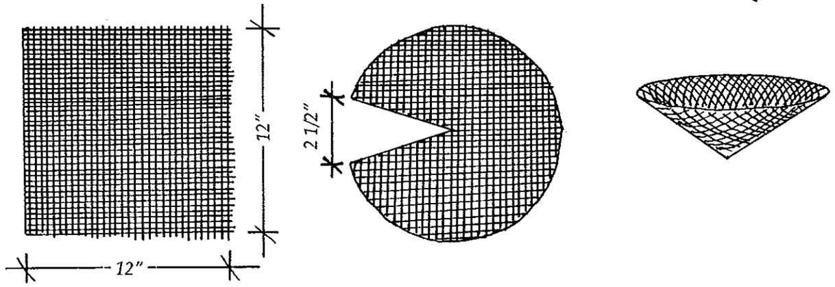
*Cut with tin snips to form a circle. Cut out a narrow pie-shape, and wire edges together to form a cone. Wire and/or staple cone into the crotch of a tree limb.*
